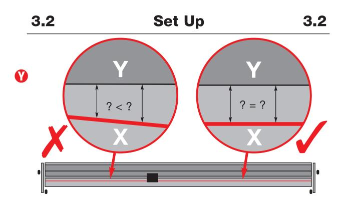
Adjust the straightness of the Base by adjusting the front "<sup>(1)</sup> and rear "<sup>(1)</sup> grub screws in the Base Fixing Brackets:
