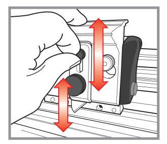
The VA (vertical action) cutting head holds two cutters which can be changed and used independently of each other. Each of the standard GRAPHIK blade holders can be set to cut at different depths and in either direction by simply adjusting or flipping the blade over in the holder. You can also push or pull the cutting head to suit your own comfort.
