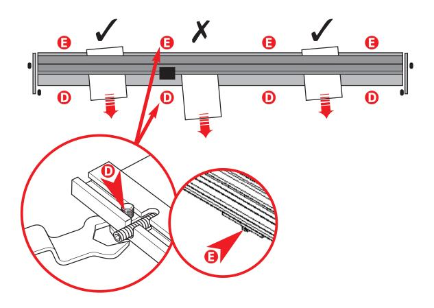
Adjust the clamping by turning the Jacking Screws "<sup>①</sup>" & "<sup>③</sup>" in the Base Fixing Brackets that are adjacent to the areas that are not clamping the paper. Turn the Jacking Screws clockwise (as you look down on them) using the wrench supplied, turn both the front and rear Jacking Screw by the same amount (to keep the Bracket level) until the paper is gripped. You may find that two or three adjacent Brackets need adjusting if you have a wide area that does not clamp.
