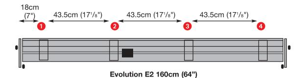
Lift the Evolution E2 cutter bar from its crate **but** <u>do not remove the clear plastic</u> <u>stretch-wrap bands</u> holding the base to the cutter bar. Place the Evolution E2 centrally on the Brackets and manoeuvre it until the base is located properly down on each of the Brackets.
